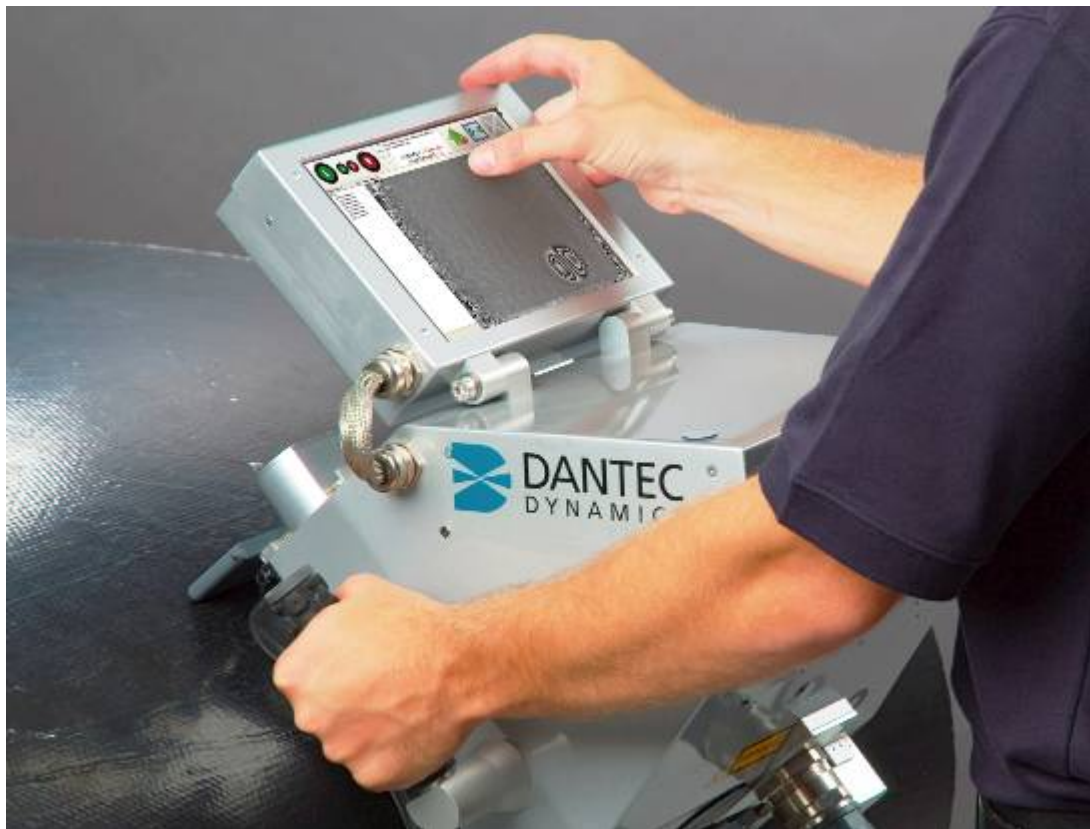
Fully integrated Q-810 Pro-line inspection system for production and in-field inspection of large surface areas
