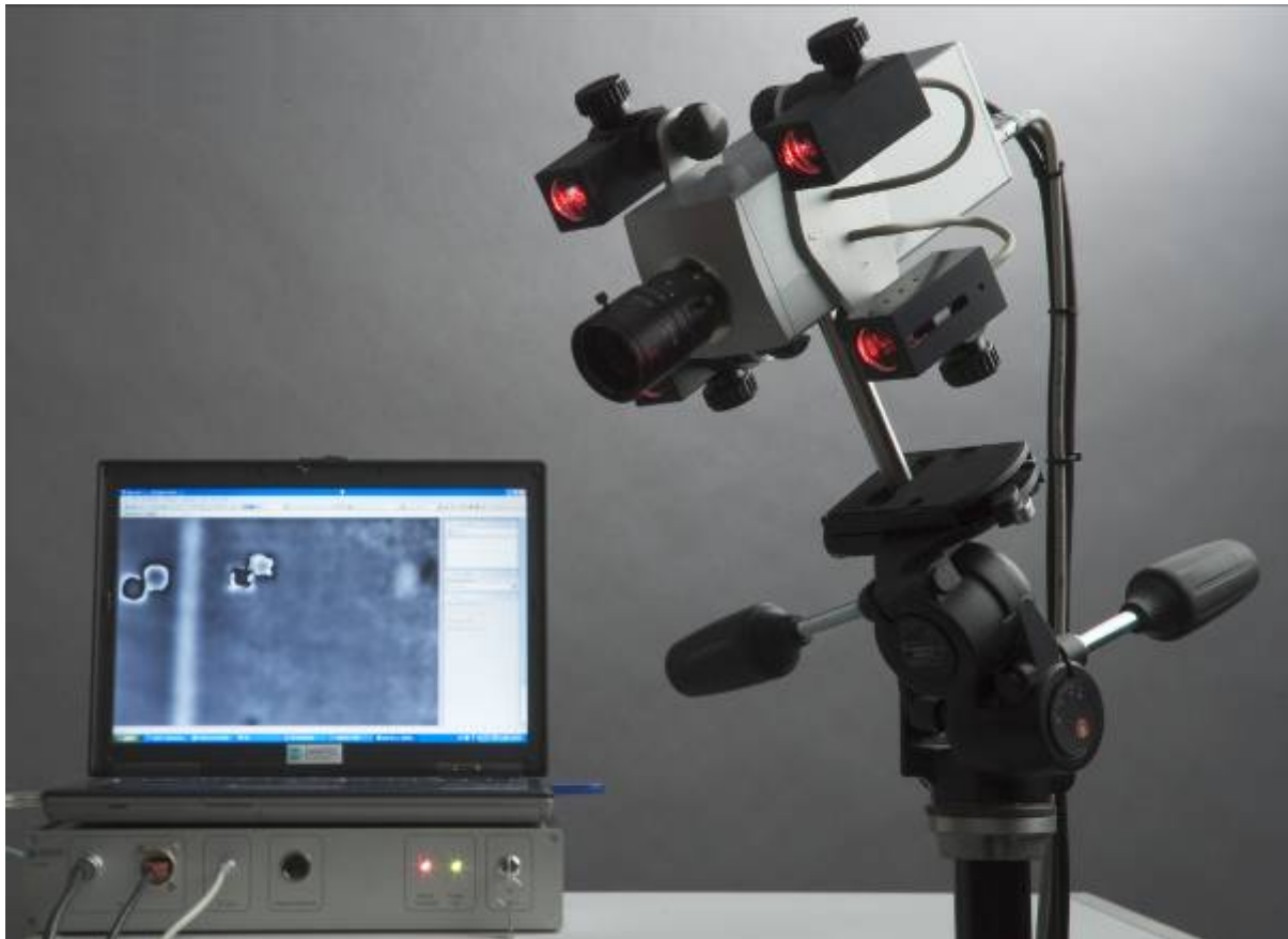
Portable Q-800 System with 4 laser diodes - Non Destructive Testing, Non-Contact, Full-Field
