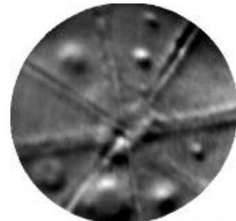
Live results from an inspection showing impact damage and structural information
